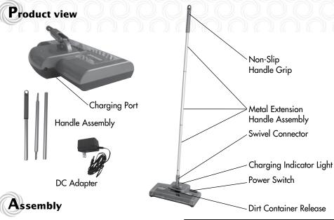
The Supreme Sweep Compact requires very little assembly. Remove it from the box and check it against the illustration to familiarize yourself with the components listed. The exploded view diagram with part names will also be helpful if you should need to order a part at a later time.
